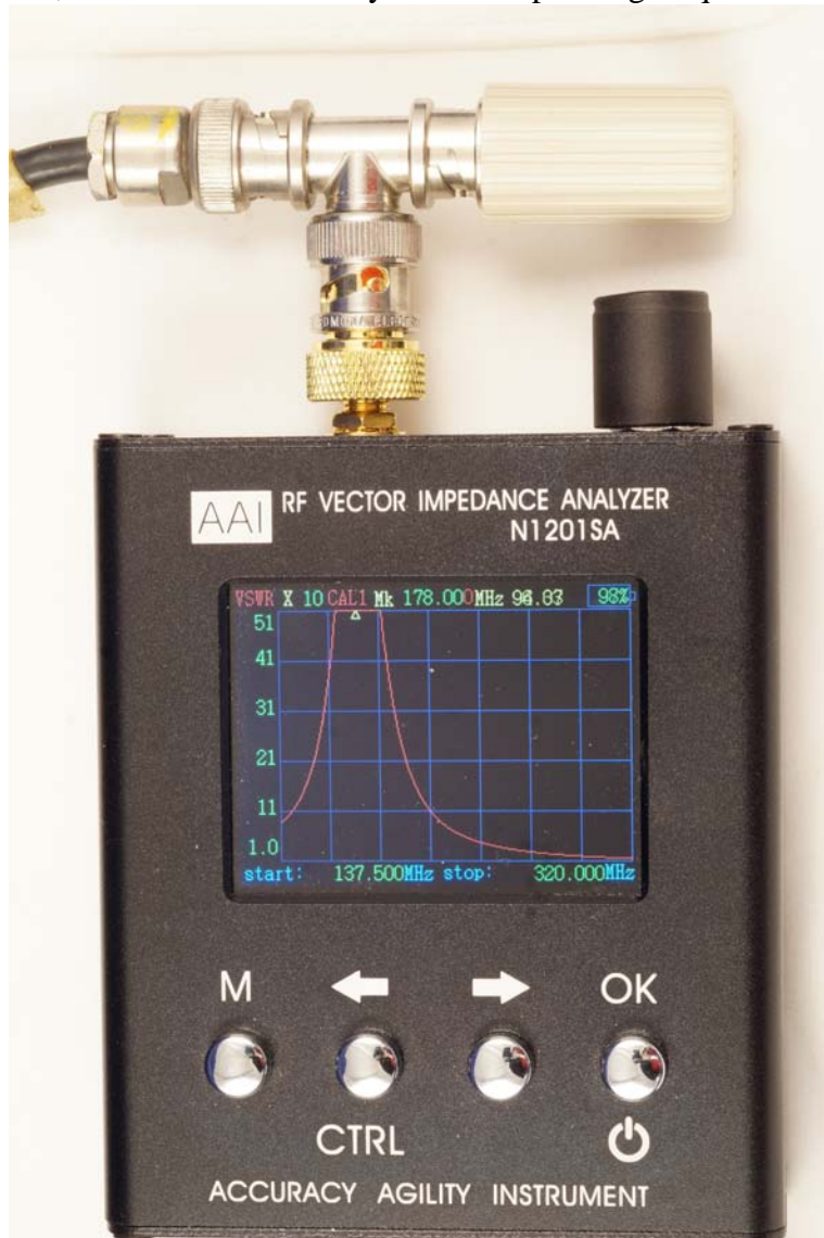
Figure 9 – Measuring resonant frequency of a stub
